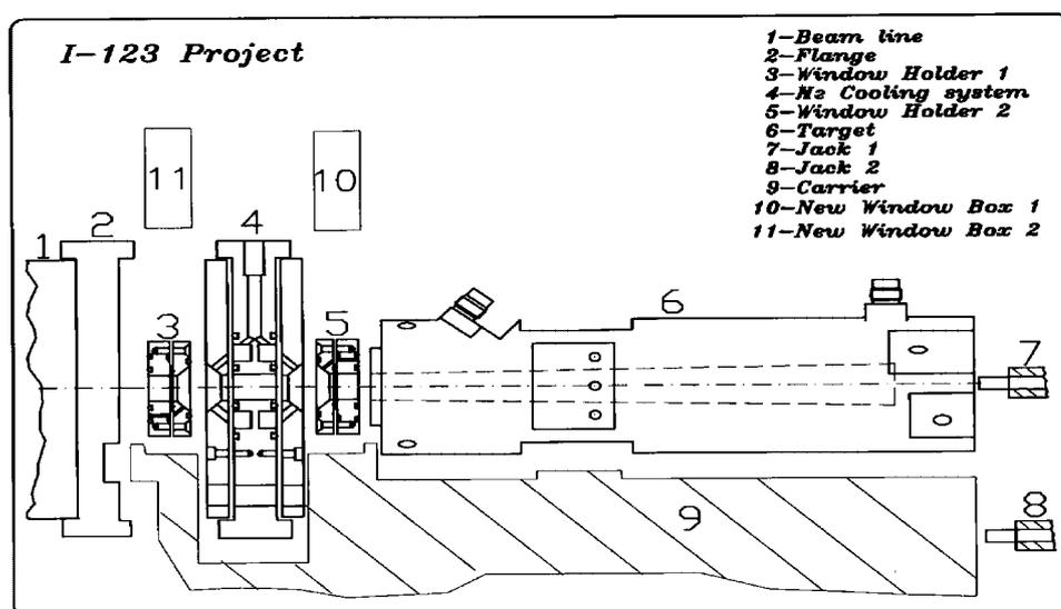
**Figure 1** Diagram of Xe-124 gas target.
